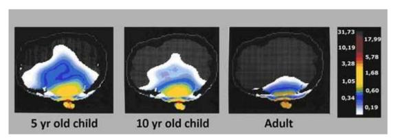
**Figure 1.** Model estimate of the absorption of electromagnetic radiation from a cell phone based on age (Frequency GSM 900 Mhz) (On the right, color scale showing the Specific Absorption Rate in W/kg) [1]
