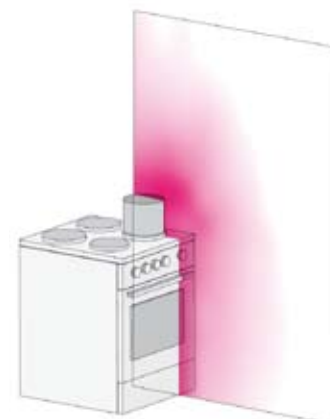
Like all appliances that consume high levels of electricity to produce heat, electric cookers (hotplates) generate intensive magnetic fields. However, the exposure quickly diminishes with increasing distance.
